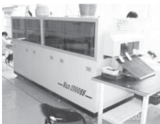
Fig. 4.6 Low residue no-clean wave solder machine at Wen'an
