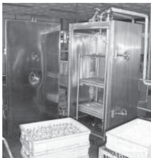
Fig. 4.4 Vacuum Drying Chamber at Cosmopolitan
