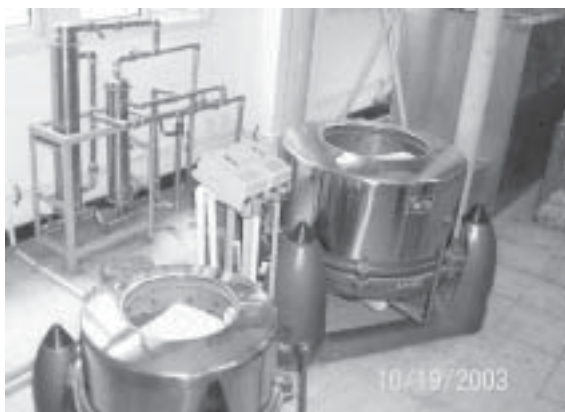
Fig. 4.9 Centrifuge dryers and water filters at Photic Plastic
