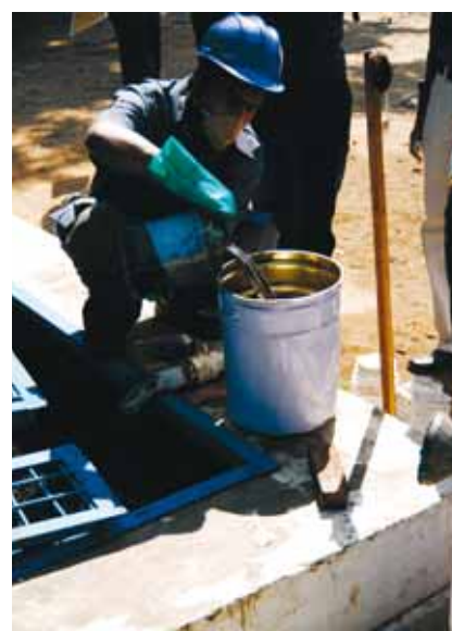
IVL collaborated with industrial companies in many different fields in Hyderabad. Process water being sampled at a factory in Hyderabad, India.
