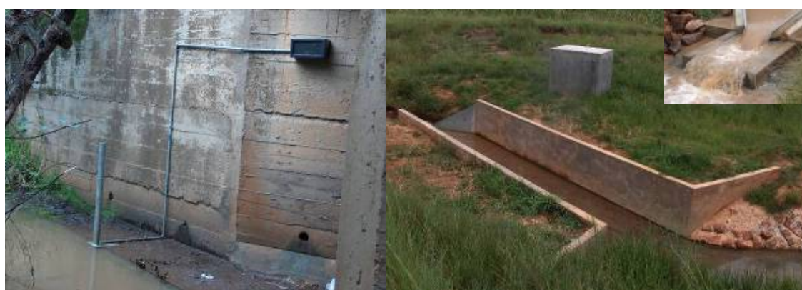
Figure 2.12: The Potshini H-Flume, and Pressure transducer at the outlet of the Potshini catchment.
