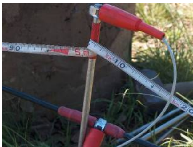
Figure 2.15: Electrical resistivity survey.
