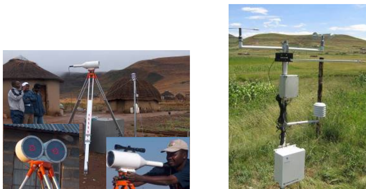
Figure 2.13: The Potshini Automatic Weather Station and Large Aperture Scintillometer.
