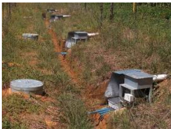
Figure 2.7: Communal trial site (researcher-managed) – runoff plots, tipping buckets, splitters and sediment load sampling tanks.
