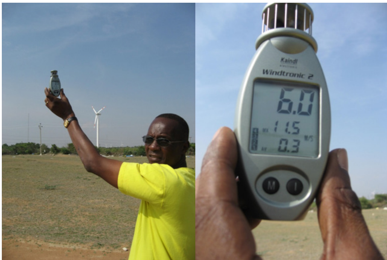
Figure 16: Wind monitoring by hand-held equipment can give a first indication of possible sites for wind projects but in order to get reliable data for designing a wind farm, wind measurements at higher altitudes and over a longer time period is needed.
